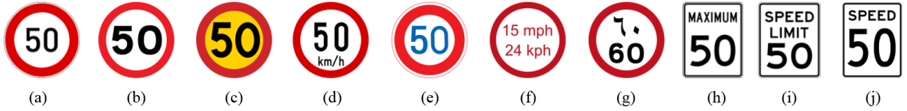
Fig. 3. Traffic sign templates for speed limits in different countries [source www.wikipedia.org ]. (a) Vienna convention. (b) United Kingdom. (c) Alternative Vienna convention. (d) Ireland. (e) Japan. (f) Samoa. (g) United Arab Emirates and Saudi Arabia. (h) Canada. (i) United States. (j) United States (Oregon variant).
